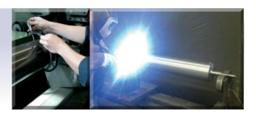
The surface is then prepared for correct size and appropriate corrosion resistance. This fresh surface is then thermally sprayed with a plasma process containing ceramic particulate.
