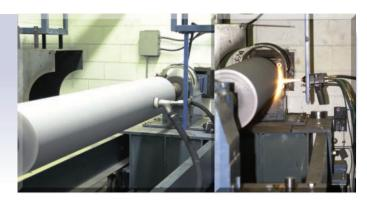
The ceramic roll is then polished to a 2.00 Ra mirror finish via a vibrating diamond head.
