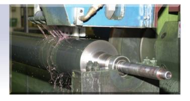
The polished roll is then mounted on the latest technological laser engraving machine, checked for a tolerance of .0002 TIR, and the roll surface is engraved to the desired specification.
